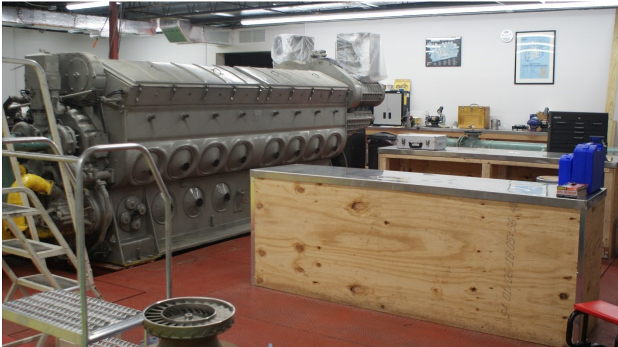
Pictured above: EMD 16-645 used for diesel engine maintenance labs
